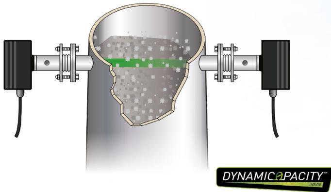
The PCME STACK 602 is a Modbus-based cross-stack optical measuring system which uses a dynamic sensing technique to measure the rate of change of light (*DynamicOpacity*<sup>®</sup> Ratiometric Opacity technology) as particulates pass through a modulated light beam.
