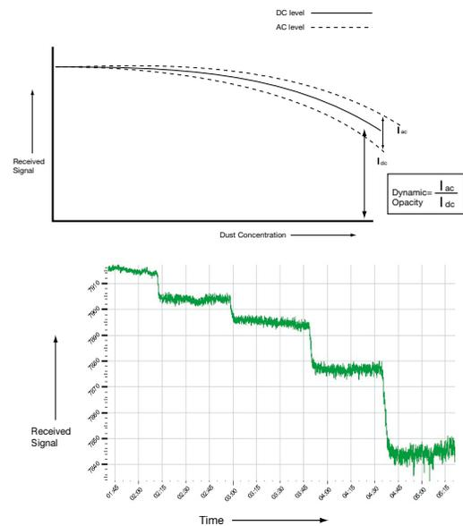
Increasing dust concentration influences Opacity and *DynamicOpacity*<sup>®</sup> Ratiometric Opacity technology
